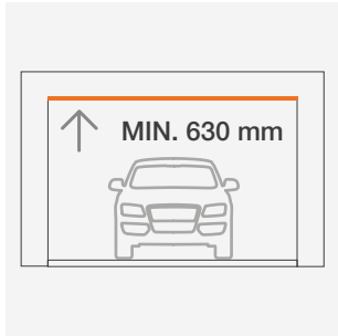
A Architrave dimension 630 mm
