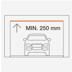
A Architrave dimension 250 mm
