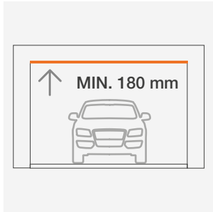
A Architrave dimension 180 mm
