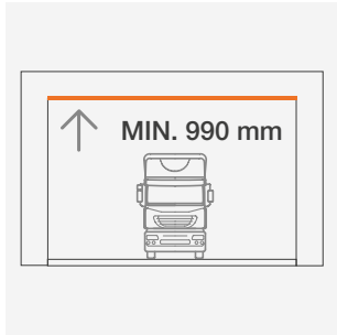
Ⓐ Architrave dimension from 990 to 4350 mm
